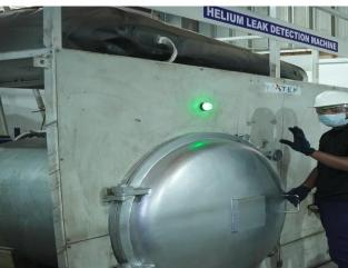
Our company specializes in providing advanced facilities for quality control and precision measurement, ensuring the highest standards across diverse industries. We utilize helium gas leak detectors to identify and locate even the smallest leaks in systems or components. Helium, with its small atomic size and inert properties, is an ideal tracer gas for leak detection, allowing us to ensure the integrity of critical products such as vacuum chambers, valves, and hermetic seals.
